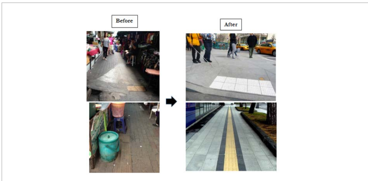
Figure 94: Concept of before and after redevelop the tactile paving and dropped kerb (Source: Consultant, 2015)
