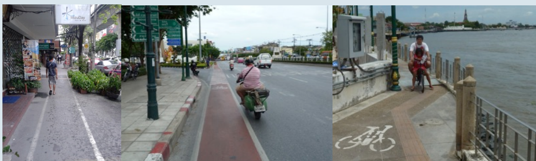
Figure 3-6: shared path (left), bike lane on the road (middle) and exclusive bike lanes (right) (Pictures: Stefan Bakker, 2014)
